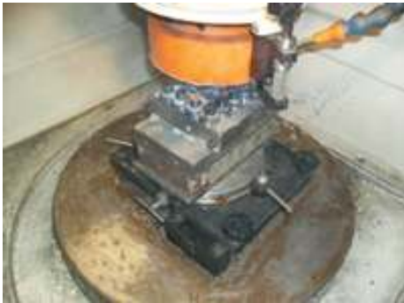
Punches, held in a gang fixture, are sharpened in a DCM grinder.
