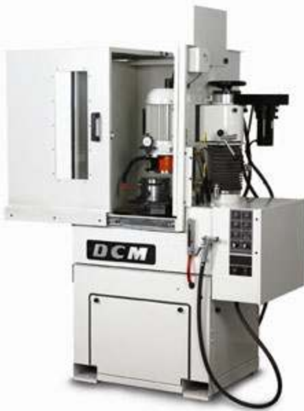
Figure 2: A full enclosure is an option for those metal fabricators looking to control mist that may emanate from the grinding process.
