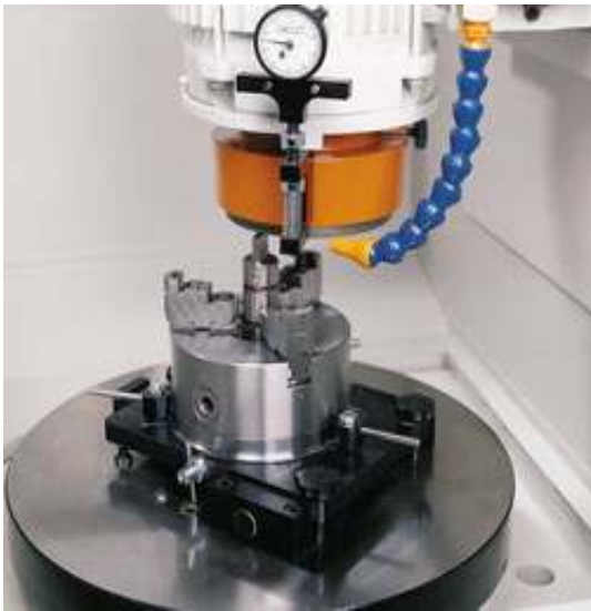
Figure 1: The vertical spindle rotary table design delivers a flat grind of punch tooling.
